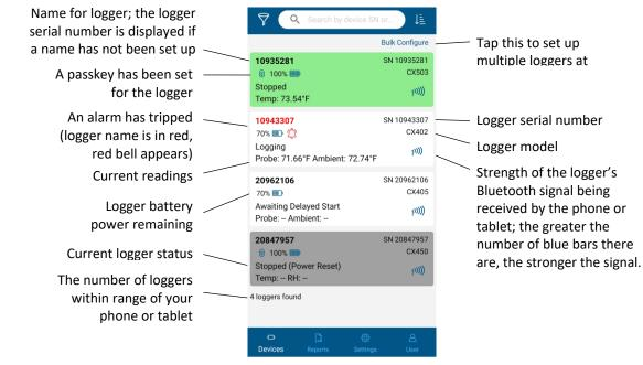
**Note for CX400 loggers:** Probe and sensor readings are displayed as "--" when the logger is stopped. "Error" is displayed if the probe is disconnected from the logger. Probe and sensor readings are updated at a different rate than the logging interval and may not match what is currently displayed on the logger LCD.
